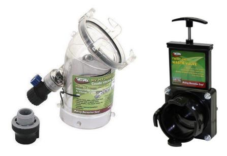
By placing the twist-on external gate valve on the end of the sewer line, you can close the valve before traveling. When setting up, attach the sewer hose before opening the external gate valve. Any waste water in the lines will go harmlessly down the sewer.
